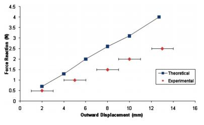
Fig. 4 Accura 25 prototype force-displacement curves
